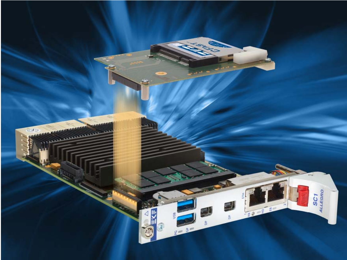
C41-CFAST over SC1-ALLEGRO CPU Card
