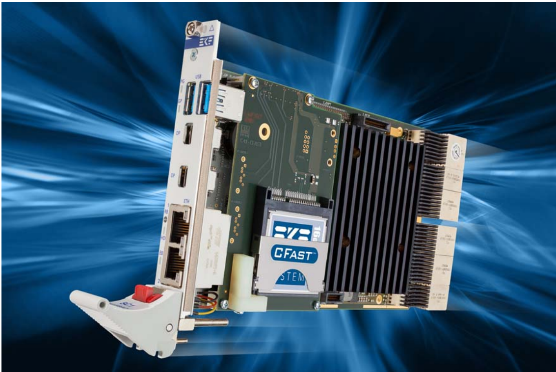
C41-CFAST on the SC1-ALLEGRO CPU Card
